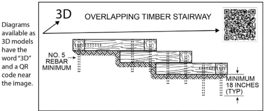
**Figure 1-1.** Some diagrams have a 3D model available; scan the QR code to access these models. More detailed diagrams of some structures and other resources are on the [Plans for Trail and Trail Bridge Structures web page](#).
