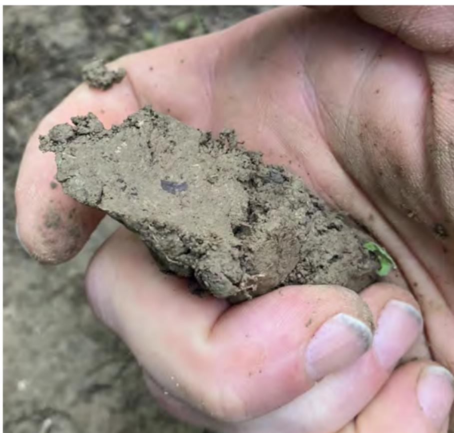
**Figure 2-9.** Clay soils hold water and swell when wet. They can create a strong tread when combined with gravel and rock. USDA photo by Matt Able.
