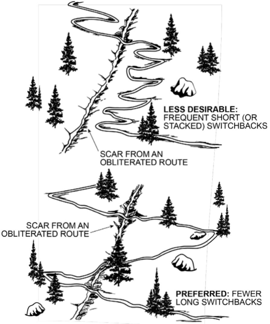
**Figure 4-31.** Long sections of trail between switchbacks are better than short sections that require more switchbacks with more opportunities to shortcut. Fewer switchbacks also means less construction and maintenance.
