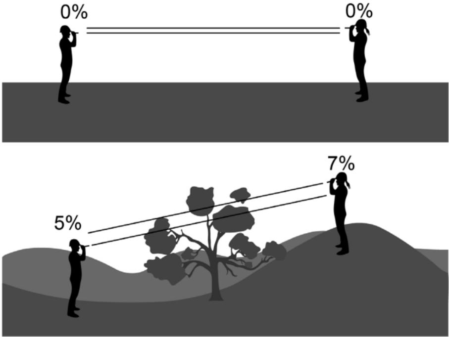
**Figure 6-4.** The easiest way to use a clinometer is with a partner. Use the steps above to determine the percent of the grade.
