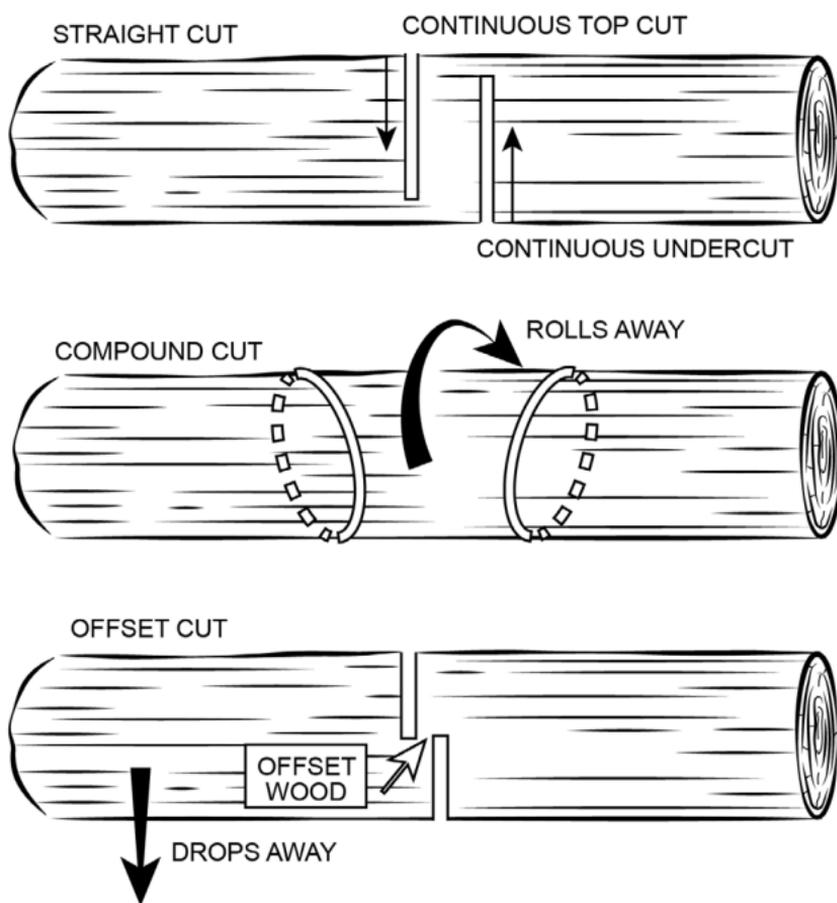
Figure 3-10. Basic log cuts for bucking logs.
