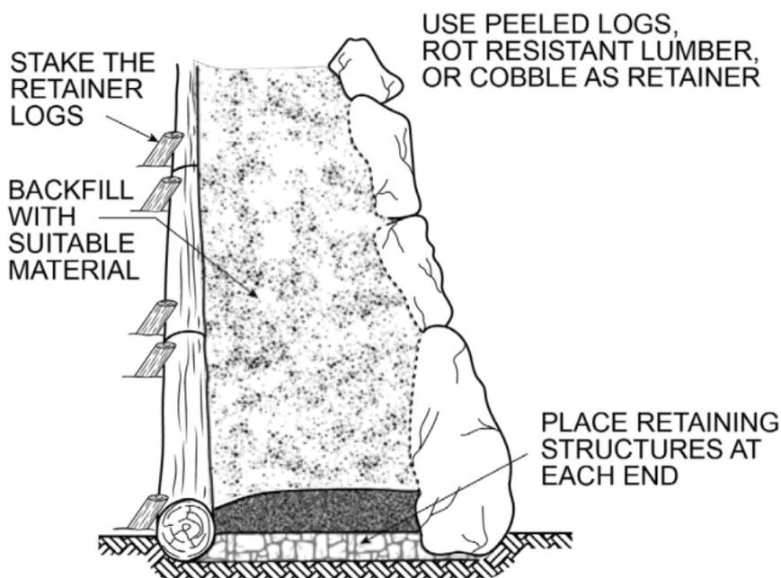
**Figure 4-11.** Causeways are turnpikes without ditches. They create an elevated, hardened tread and are best used across seasonally wet areas or to cover and replace multiple parallel paths. Diagram based on [Forest Service standard trail drawing](#) STD 932-20-01.
