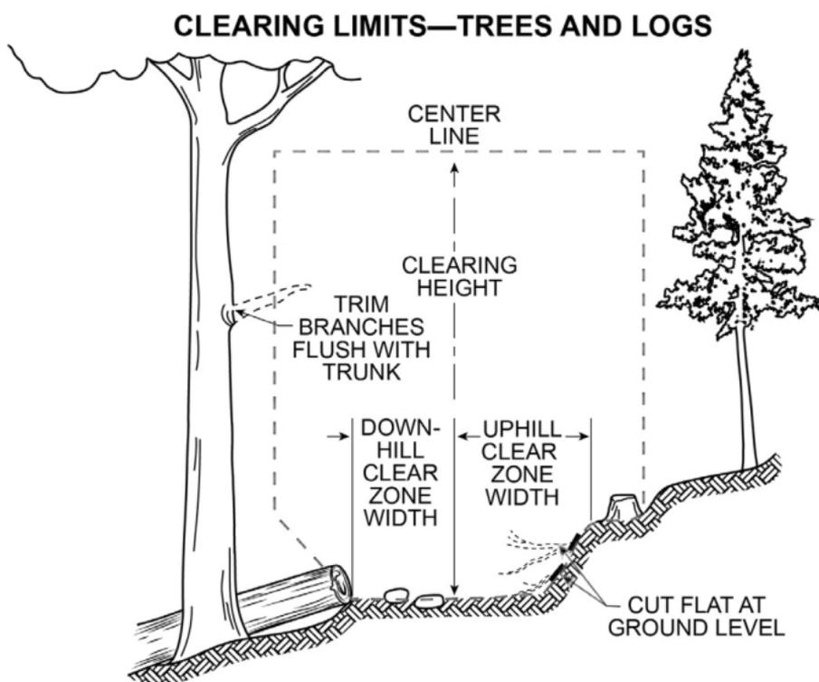
**Figure 3-2.** Corridor clearing height and uphill and downhill clearing widths differ depending on the type and development scale of the trail. Diagram based on [Forest Service standard trail drawing](#) STD 912-01.
