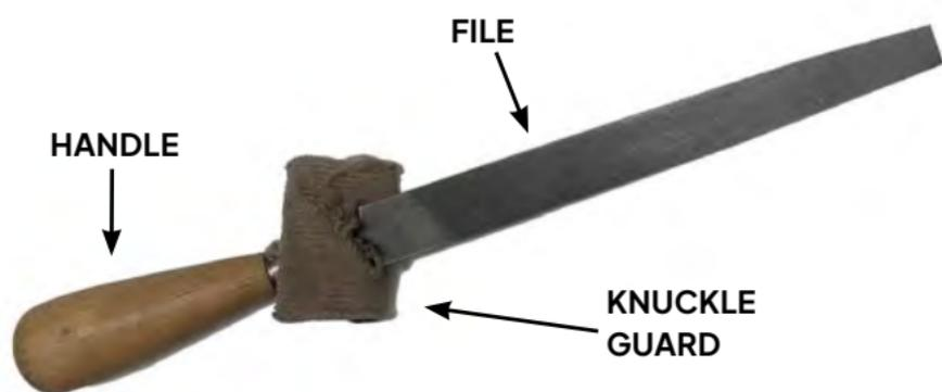
**Figure 7-24.** A hand file with a handle and a knuckle guard made from an old fire hose. USDA photo by Kerry Wood.
