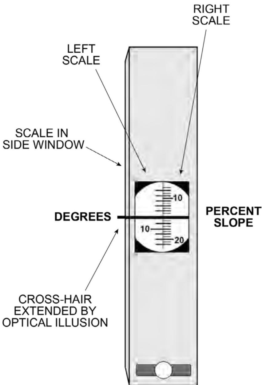
Figure 6-3. Diagram of a clinometer.
