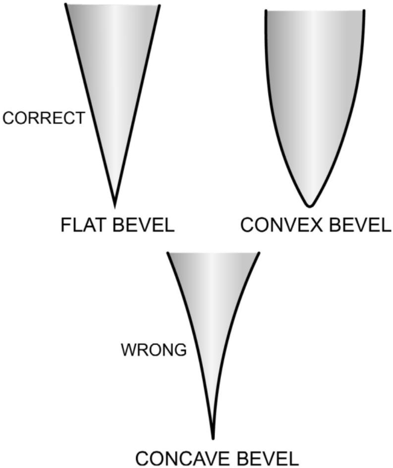
**Figure 7-23.** Illustration of correct and incorrect blade bevels.
