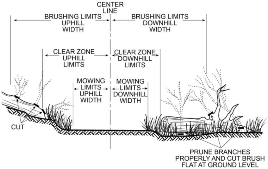
**Figure 3-5.** The trail corridor clearing dimensions change depending on the trail type and development scale. The clearing dimensions for each trail are documented in the TMO. Diagram based on [Forest Service standard trail drawing STD 912-02](#).
