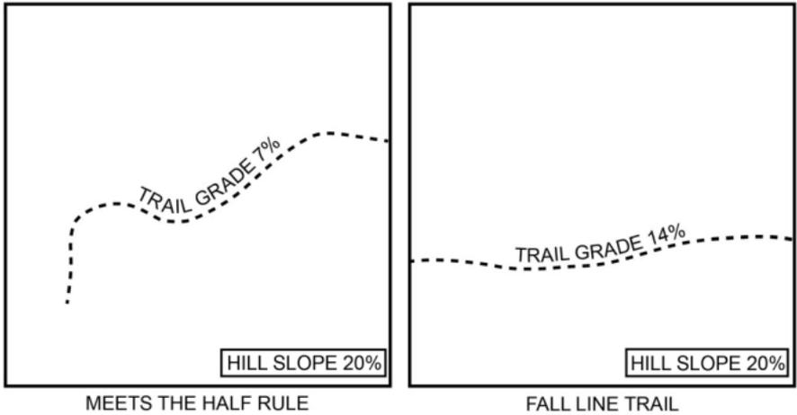
**Figure 2–24.** Plot a trail on the map with the half rule in mind. Trails with grades less than half of the prevailing hillside slope meet the half rule and will generally be more sustainable. Trail grades more than half of the prevailing hillside slope are fall line trails, will generally be prone to erosion, and require more frequent maintenance.
