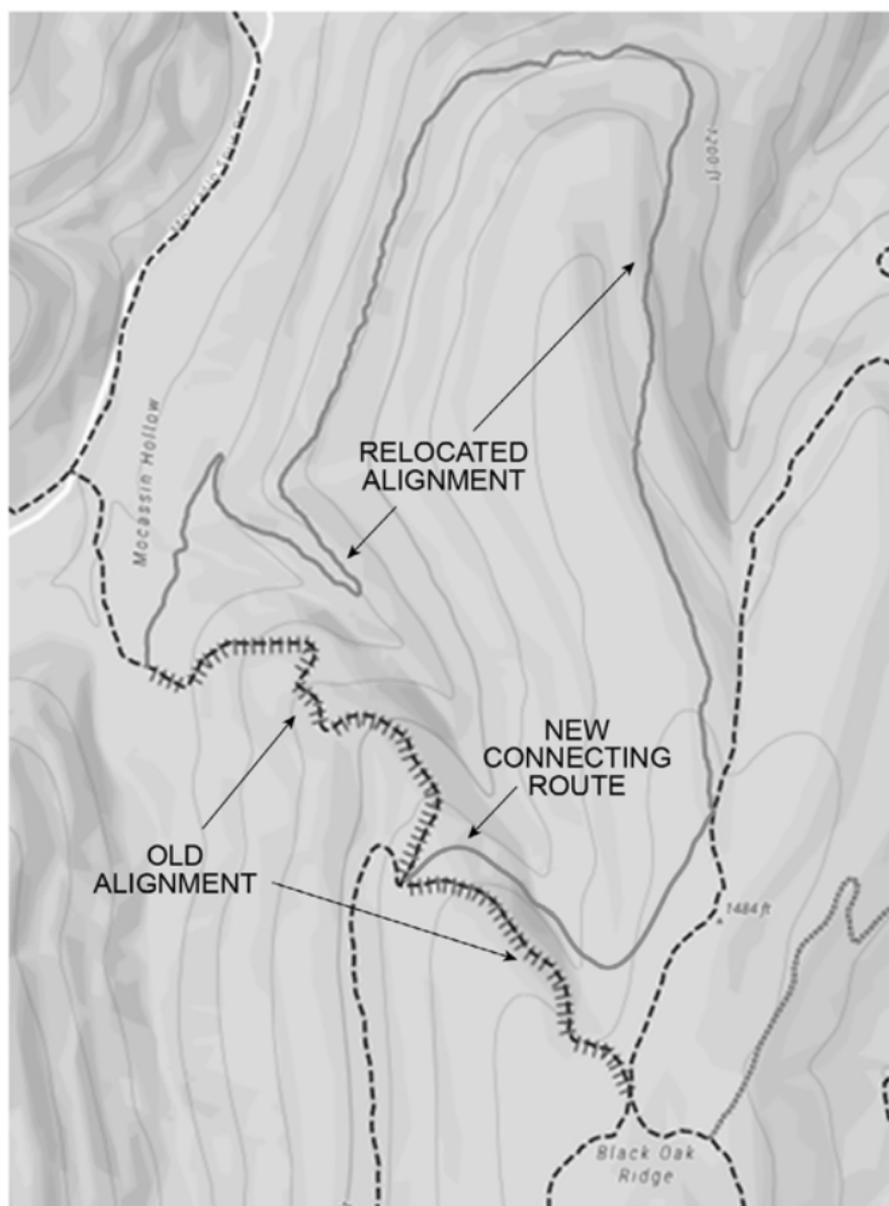
**Figure 6-1.** Trail relocations are often double (or more) than the length of the segment of trail they are replacing to allow for lower average grade, sufficient grade reversals, and other physically sustainable design elements.
