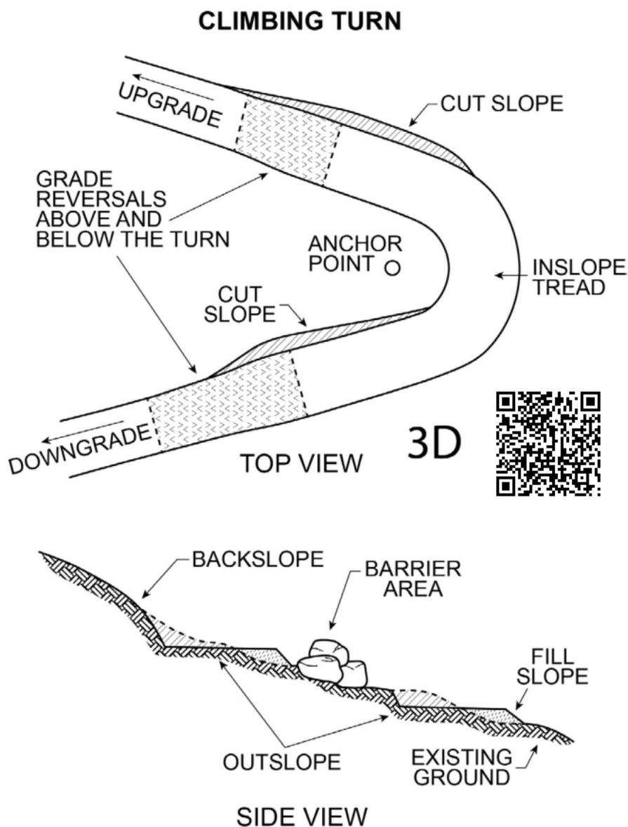
**Figure 4–29.** Climbing turn. Diagram based on [Forest Service standard trail drawing STD 914–01](#).
