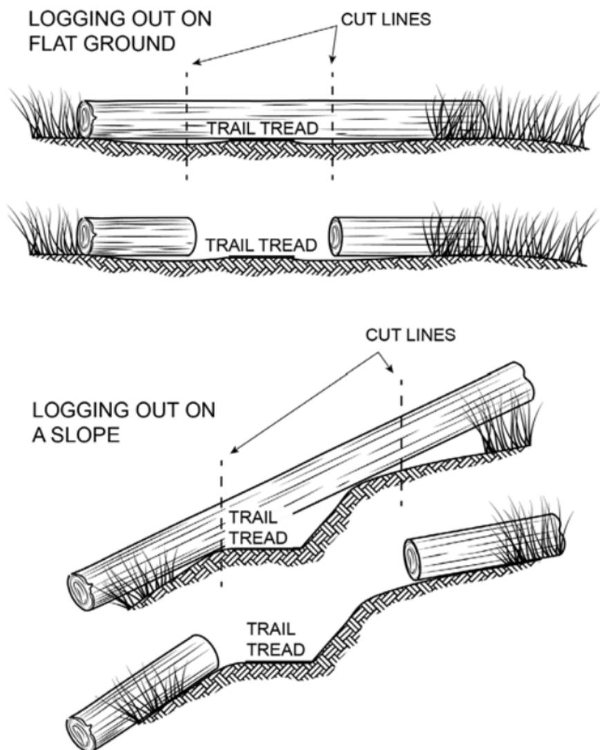
**Figure 3–8.** Clearing limits can change as the slope increases, particularly on trails open to motorized uses.
