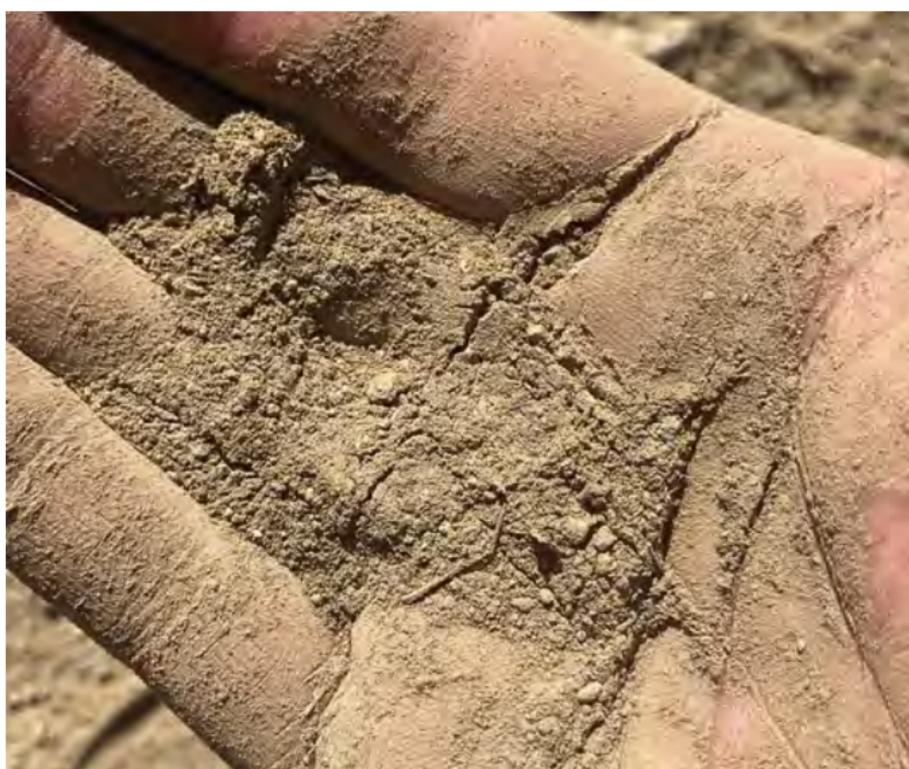
**Figure 2-8.** Silty soils hold water when they are wet and are floury when dry. They are best suited for trail building when mixed with gravel and rock. USDA photo by Matt Able.
