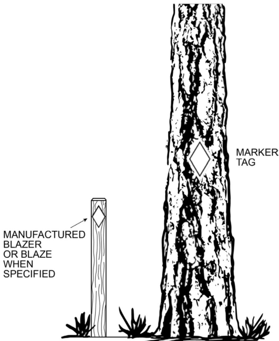
**Figure 5-6.** Most trail managers use reassurance markers nailed to posts or trees. Blazes are no longer cut into trees in many parts of the country. If it is still a practice in your area, blaze the tree on both sides. Cut the blaze no deeper than needed for clear visibility. Diagram based on [Forest Service standard trail drawing STD 953-01](#).
