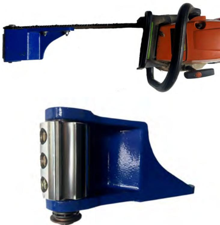
**Figure 7–18.** Chainsaw debarking attachment.
