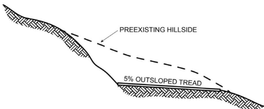
**Figure 6-9.** Construct a full-bench trail by cutting the full width of the tread into the hillside. Outslope the tread 3–8 percent (or maximum 5 percent on trails designed for accessibility). Diagram based on [Forest Service standard trail drawing](#) STD 911-01 (A section).
