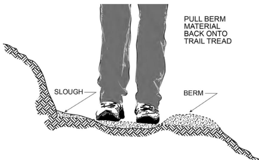
**Figure 3–13.** Remove the slough and berm, leaving the trail outsloped so water will run off.
