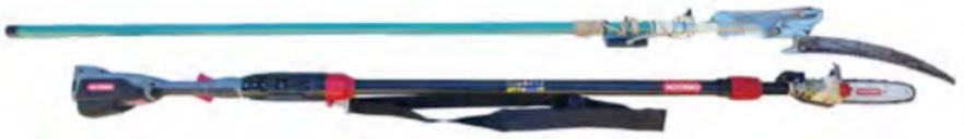
**Figure 7–30.** Manual pruning saw (top) and electric pruning saw (bottom). USDA photo by Scott Johnson.
