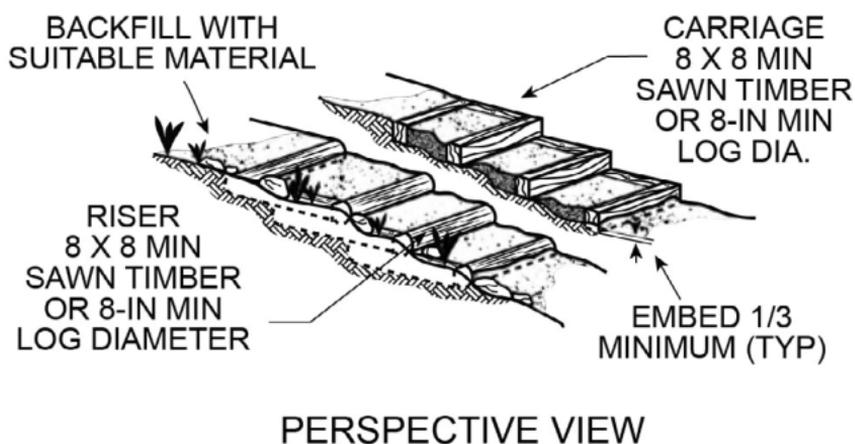
**Figure 4-53.** Side and perspective view of overlapping timber stairway. Diagram based on [Forest Service standard trail drawing STD 936-20-02](#).
