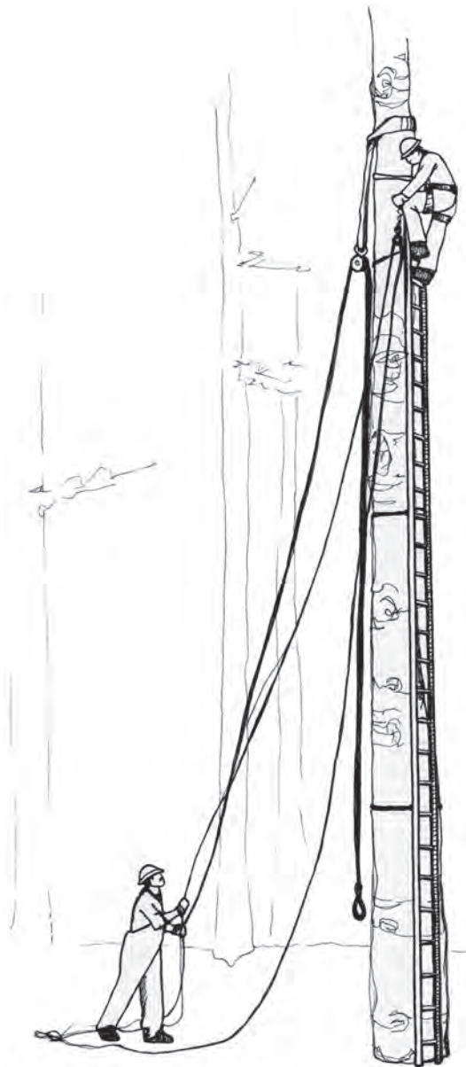
Figure 8-1 — Riggers using a sectional tree climbing ladder.
