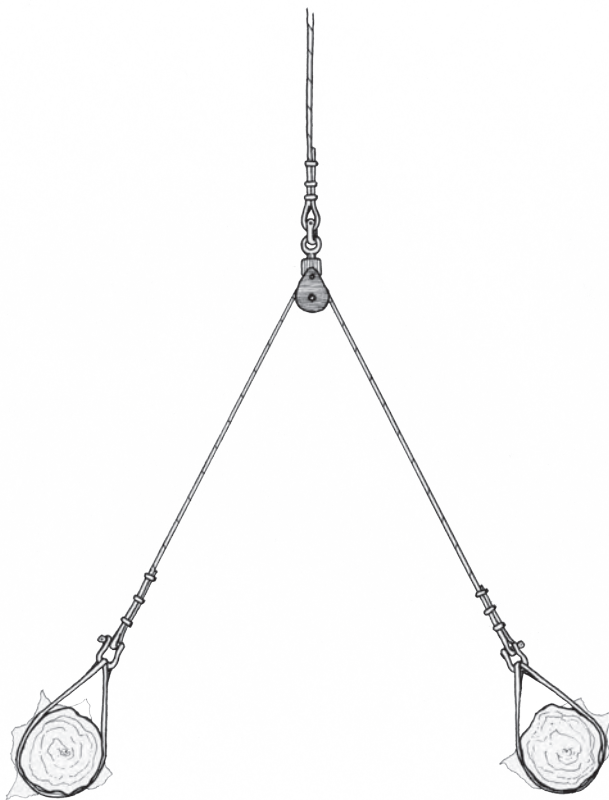
Figure 11-1—A line with multiple anchors terminating at a bridle block.
