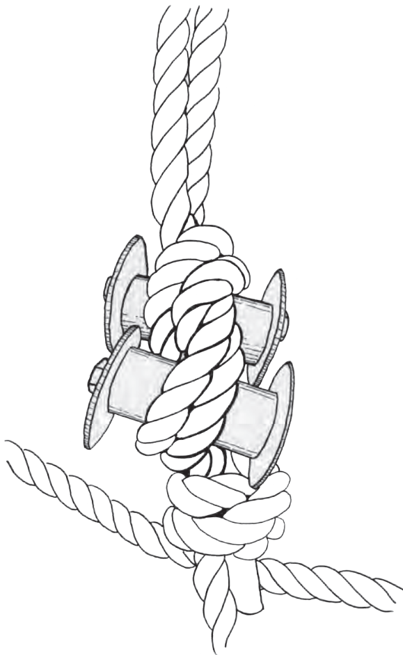
Figure 3–6—Using polyvinyl chloride pipe and washers to facilitate untying a “figure 8” knot.
