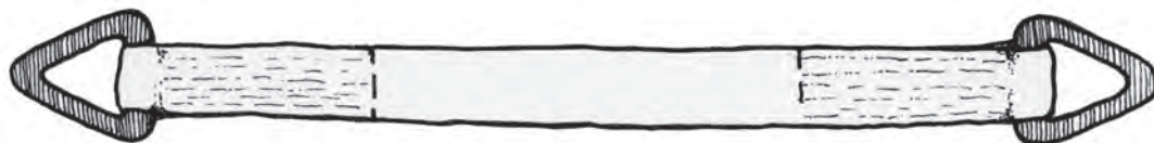
Figure 5–2—A basket-hitch nylon flat sling.
