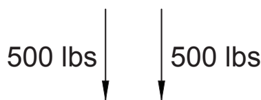
Figure E-8—When all lines are parallel in a direct pull, no force is lost in a lateral vector.
