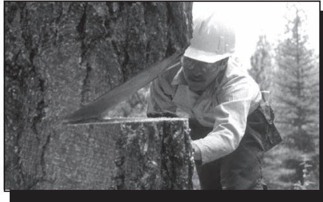
Figure 4-23—The sloping cut is a 45-degree angle.
