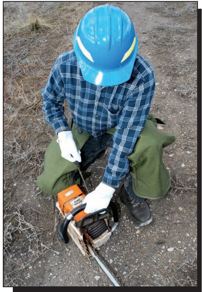
Figure 3-17—Start the saw on firm ground.
