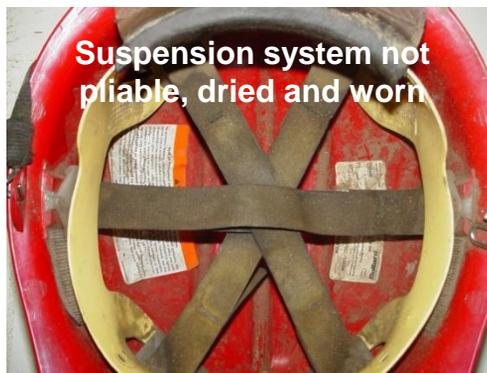
**With exception of face and neck shrouds, as shown here, inserting materials between the shell and suspension system is prohibited.**
